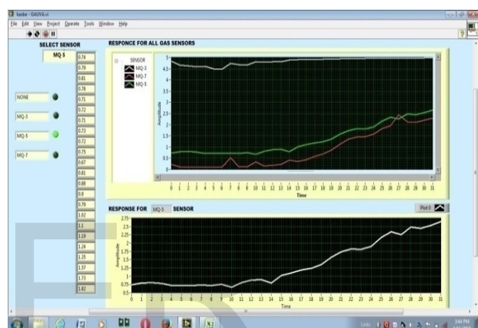
Figure9. Front panel showing gas sensor response for guava (in volts): (MQ-5)
