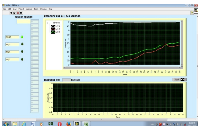
Figure7. Front panel showing sensor response for guava (in volts): (no gas sensor selected).
