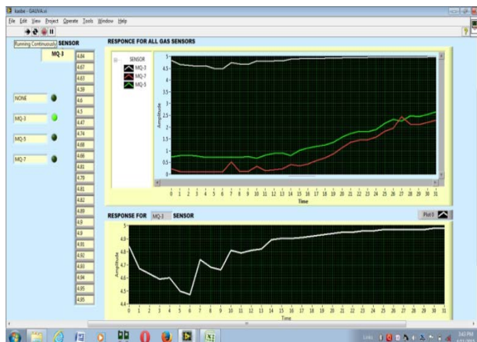
Figure8. Front panel of showing gas sensor response for guava (in volts): (MQ-3)
